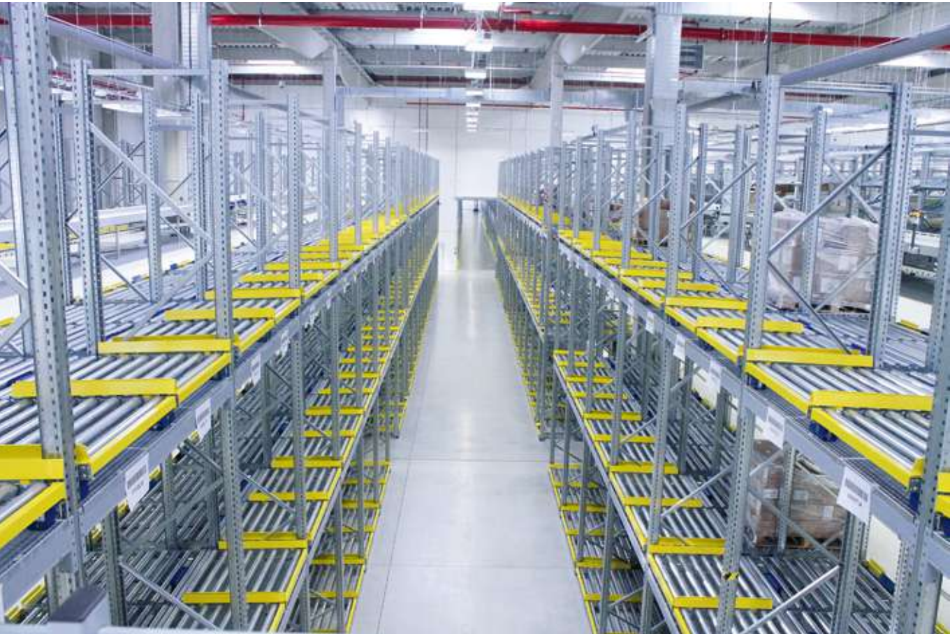
Picking roller tracks
